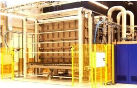
*Aston Foods Continua(r). Continuous Vacuum Cooling System for baked goods. Cooling time for tin bread: 3 minutes. Capacity 6500 bread loaf/hour. Footprint 18 square meters. / Further text by ots and under [www.presseportal.ch](http://www.presseportal.ch). The use of this picture is for editorial purposes free of charge. Publication under source: "ots.photo/Aston Foods AG".*
